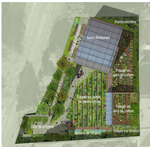
Figure 11. La Ferme du Rail is a small circular urban economy city block in the centre of Paris. The plan indicates the mixed programme fits into merely 1800 sqm. Image: Clara Simay Architect
